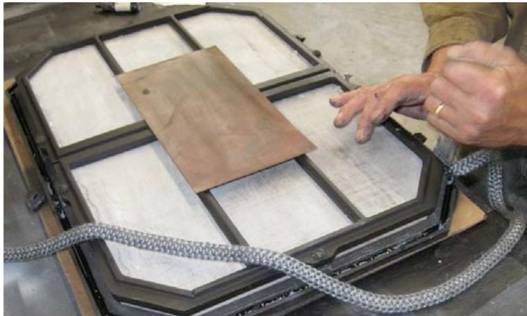
6. Allow the glue to set up for 15 minutes before placing the lid back on the stove. After waiting return the lid to the stove. Be sure the lid is properly seated on the top frame. Keep lid closed for 24 hours.
