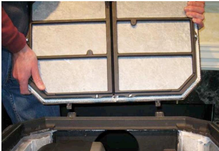
3. Use a putty knife to remove the old gasket. Remove any residual gasket and glue with a wire brush and vacuum.
