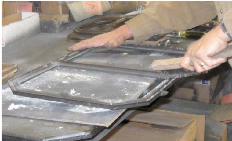
4. Dry fit the new gasket into the gasket channel. Start with one end of the gasket at the center, rear of the top lid. Press the gasket into the channel firmly all the way back to the starting point. Do not stretch or compress the gasket as you work it around the lid. Use sharp scissors to cut gasket to the proper length.
